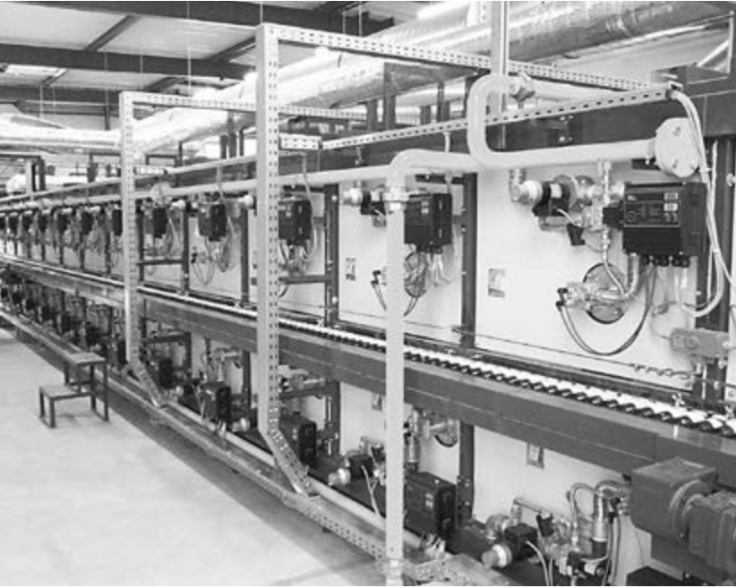
Roller hearth kiln in the ceramics industry
