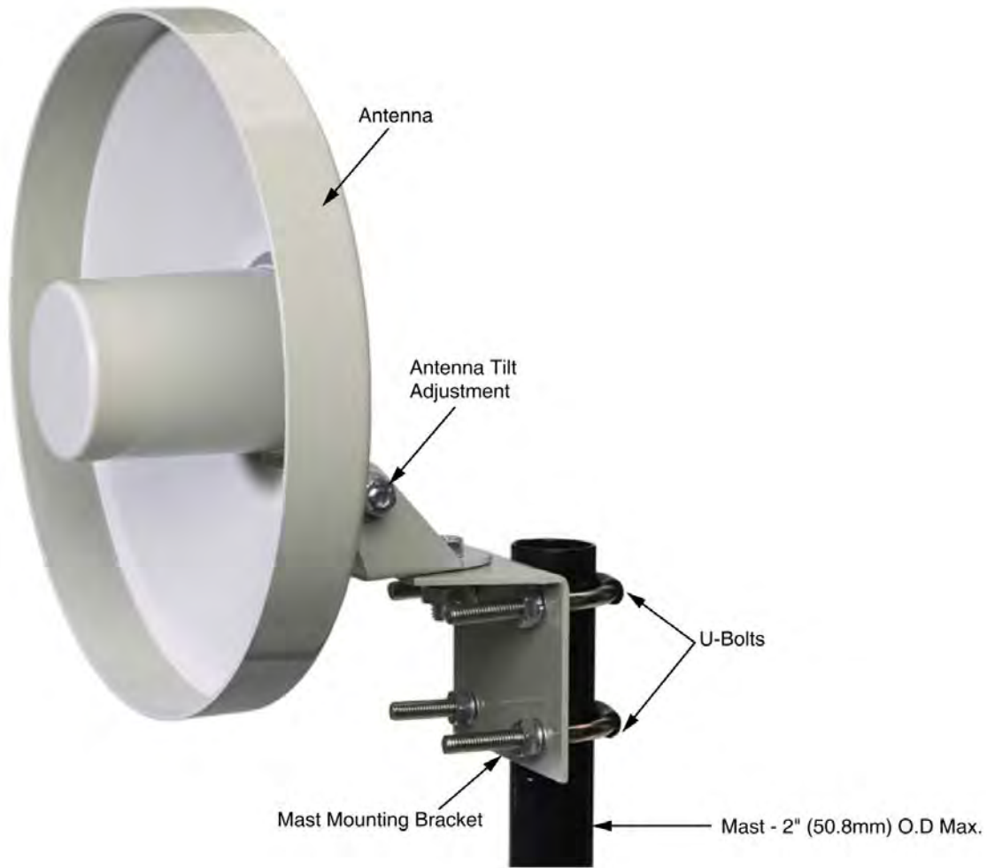
Figure 4-3 Directional antenna mounting
