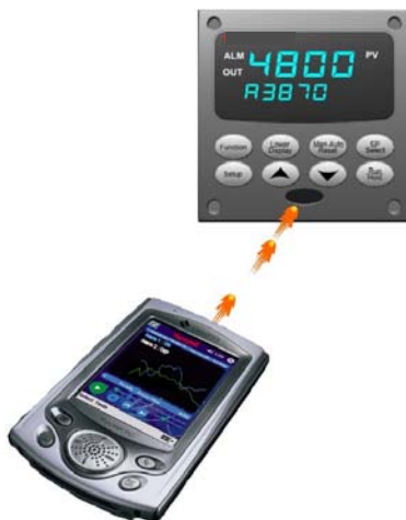
Figure 1-3 Depiction of infrared communications
