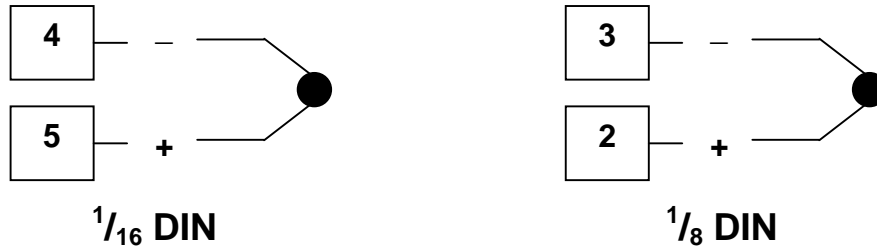
Figure 15. Thermocouple Input Connections
