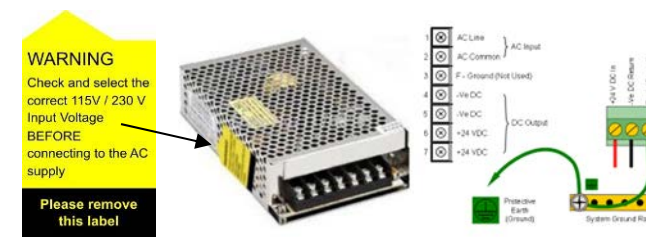
Figure 4. Switched Mode Power Supply (SMPS) Connections
